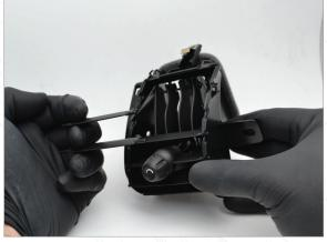
Remove the top 2 horizontal slats from the housing. NOTE: be sure to leave the linkage connected to the lower 4 horizontal slats.
