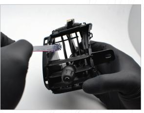
Feed the display cable through the opening on the left side of the vent as shown.
