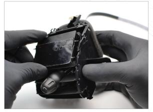
Position your display so that the bracket lines up with the slots where the top two slats originally were. Be sure that bracket is fully seated back into slots.
