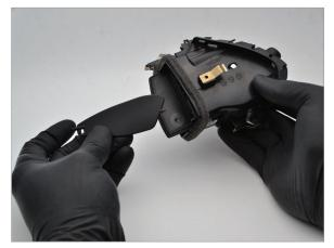
Remove the left most vertical slat from the rear of the housing.
