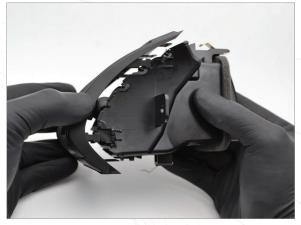
Line up the 8 tabs on the trim with the housing and fully seat the trim onto the housing.
