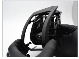
Release the 8 tabs holding the trim to the front of the housing and remove the trim.
