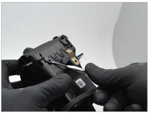
Release the bottom of the left-most vertical slat and push it toward the rear of the housing.
