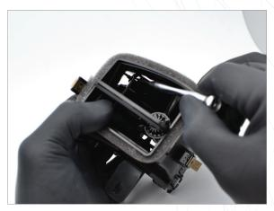
Disconnect the left-most vertical slat from the linkage. NOTE: be sure to leave the linkage connected to the other 3 vertical slats.
